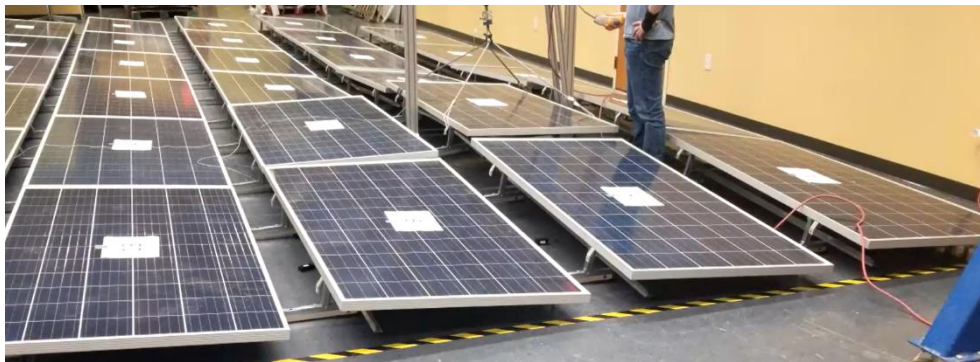
clawFR 10 Degree vertical load sharing test setup
