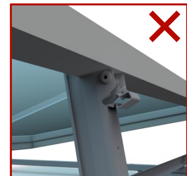
LOCK CLAW NOT INSTALLED
